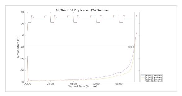
The International Safe Transit Association (ISTA) 7D Summer profile is a 24 hour stepped thermal exposure between  $+22^{\circ}$ C and  $+35^{\circ}$ C.
